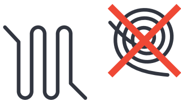
Figure 2.1 Recommended way to handle excessive cable length.
