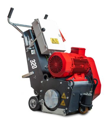
Ferox 320 World Series is a very powerful machine for both milling and shaving. Depending on the choice of tools, you can adapt the areas of use, from removing of concrete asphalt, coatings to road markings. The different tool options are designed to remove the hardest applications, coatings and floors. By using the 300 mm variable diamond drum blades, it allows for cutting depth of 2mm in a single pass. Use "cutter drum or "milling drum" for effective scarifying.
