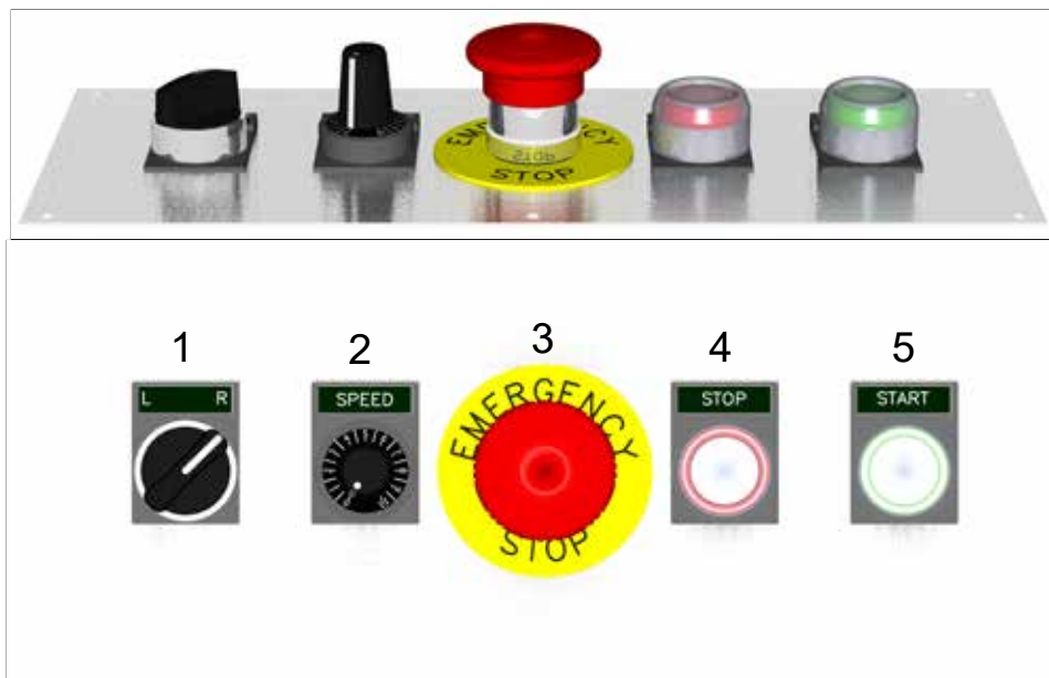
Figure 42 Control panel of Scan Combiflex 500.
