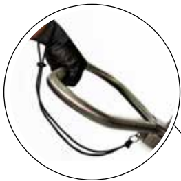
The dead man's switch replaced with a key
