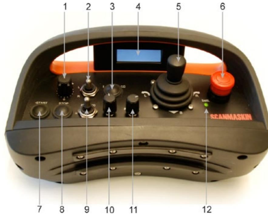
Figur 4-2 Fjärrkontroll SC-1000RC
