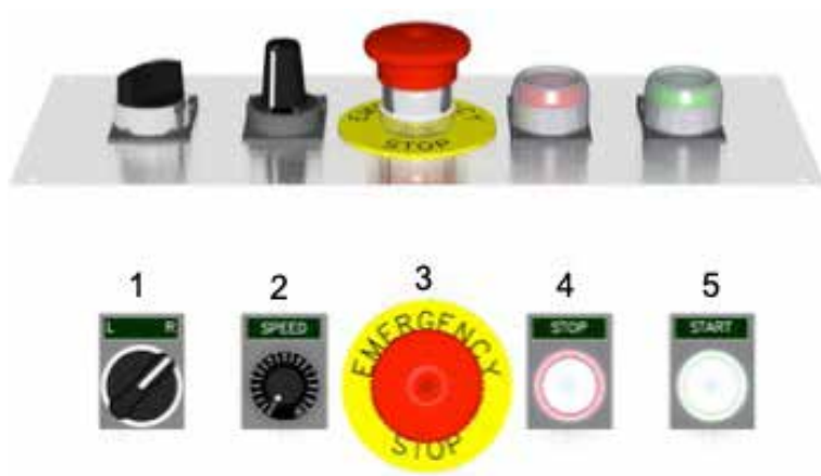
Figure 4.2 Control panel for Scanmaskin 450NS.
