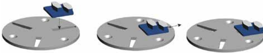
Figure 4.3 How to fit the diamond segments on the Scan-On plate
